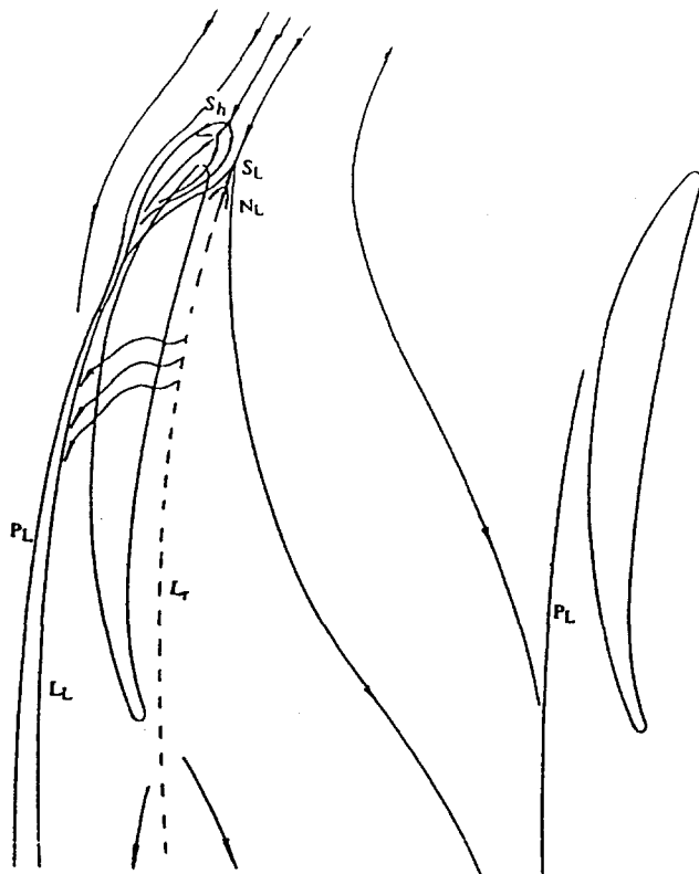
Fig. 4 Schematic of the flow pattern on the wall for 2.0 percent clearance, from Kang and Hirsch (1993a)
